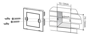
Fix screws: Use the screws supplied to attach unit to backbox using a flat head screwdriver
